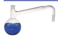
**General Distillation Apparatus and Moisture Test** KIMAX® apparatus is used in general purpose distillation and phenol distillation. The flask has a flat bottom and a distillation head with a 19/38
