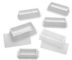
**Polystyrene Reagent Reservoirs** Trough-within-a-trough design to recover the "last few drops".
